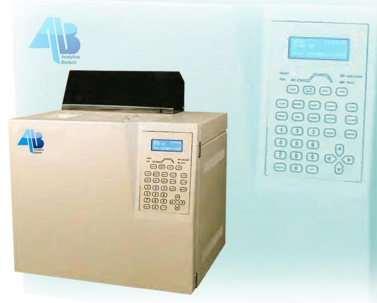
5 Independent Heated Zones up to 400° C for individual control of Injector, Detector and oven
